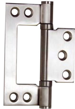
BUTT HINGE "FLUSH" 100 X 70 X 2,5 MM Item No. 15.20.100 Incl. CSK SS-304 screws Ø5 x 30 mm
